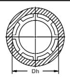
Inside Diameter With Section B-B
