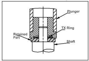
A cylindrical plunger can be easily made to install TX, TY rings. The ring is positioned at the opening of the plunger and then pushed or tapped onto the shaft, as illustrated.
