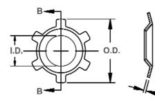
Free Diameter & Ring Measurements With Section B-B
