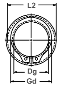
Clearance Diameter & Gaging Diameter Released in Groove.
