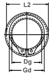
Clearance Diameter & Gaging Diameter Released in Groove.
